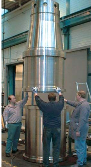
Assembly of a drum body with diameter 1,000 mm
