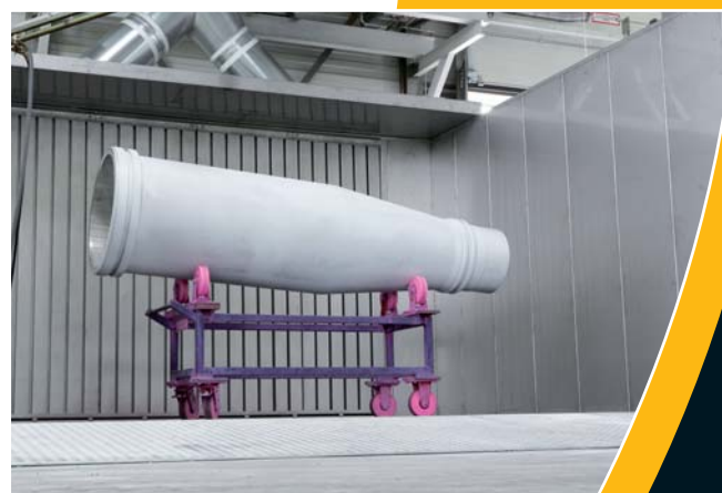
Decanter component during non-destructive inspection
