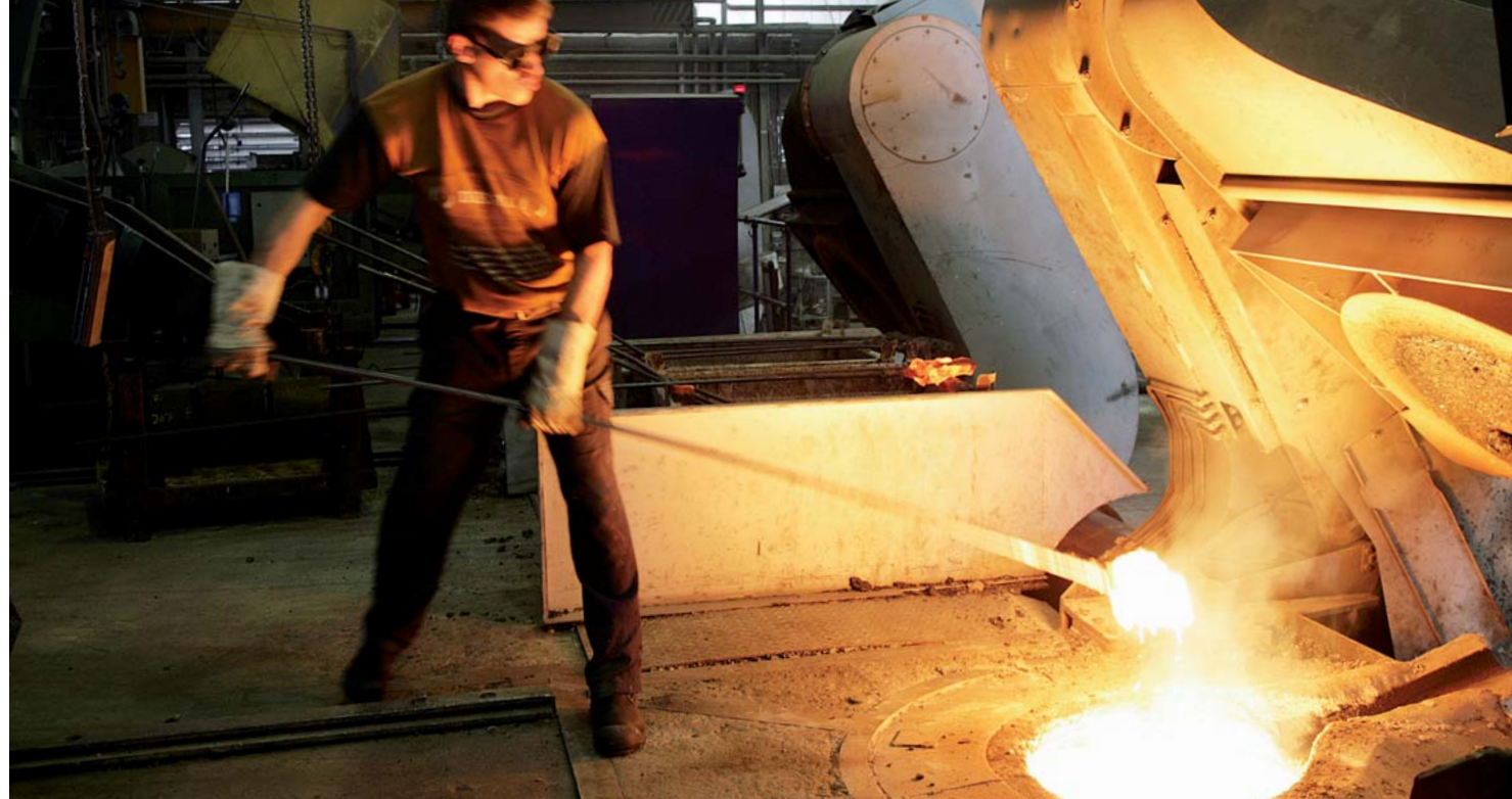
Removing a sample from the induction furnace
