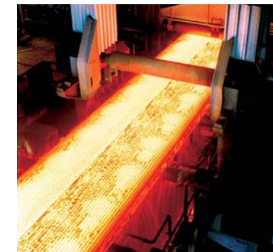
Extrusion casting rollers are produced at Kuhn Special Steel with composite centrifugal casting
