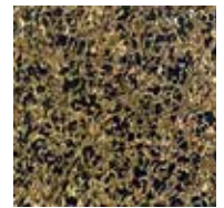
Fig. 3: Ferrite-carbide microstructure of GL21.
