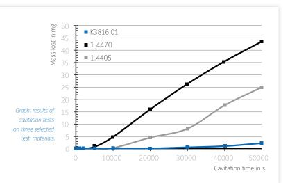
Cavitation occurs when gas-bubbles form in a flowing liquid. These bubbles are created by local pressure differences, which are in turn caused by the flow properties and gas pressure of the fluid concerned. A change in these pressure conditions leads to instability causing the bubbles to implode. If this occurs near the wall surface, a sudden impulse of pressure (known as a microjet) is directed on the surface. This short cyclic impulse can amount to several hundred MPa.
